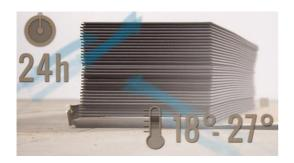
Installations in areas colder than recommended will influence the installation properties of Moduleo Dryback. The planks or tiles will be less flexible, cutting will be harder and small pieces difficult to cut out. The lower the temperature, the more difficult the installation. For installation in areas warmer than recommended, we advise consultation with your local retailer/ installer on how to create the appropriate installation conditions.
